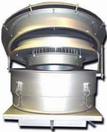
*Retrofitting a PM10 high volume air sampler allows for characterization of PM2.5 with existing methodologies.*
