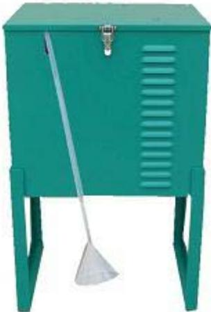
The RAC 3-Gas Sampler is a wet-chemical system that samples ambient air for up to three different pollutant gases simultaneously and features a thermoelectric system to assure maximum accuracy for SO<sub>2</sub> sampling.
